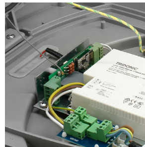
Control card imbedded in the body of the fixture
